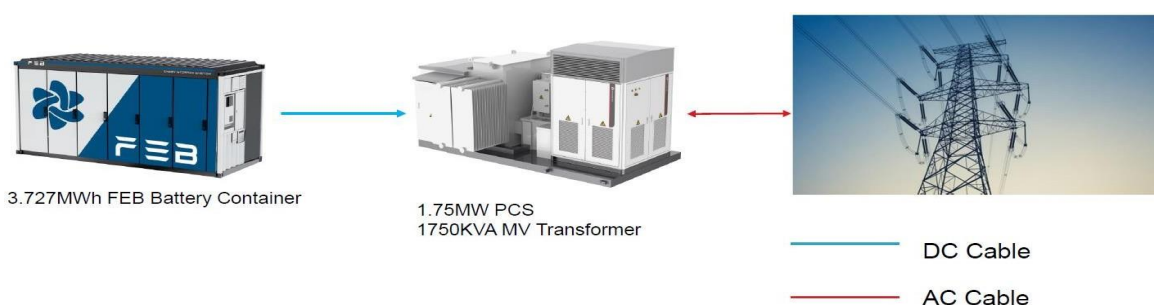
One 1.75MW/3.727MWh BESS Block
